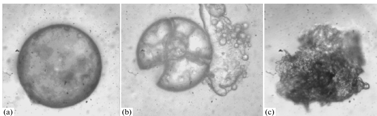
Fig. 3. Microphotography of hydrolytic degradation of biopolymer POB-based microspheres with encapsulated chlorambucil (optical microscopy): (a) 1 day, (b) 15 days, and (c) 30 days.
